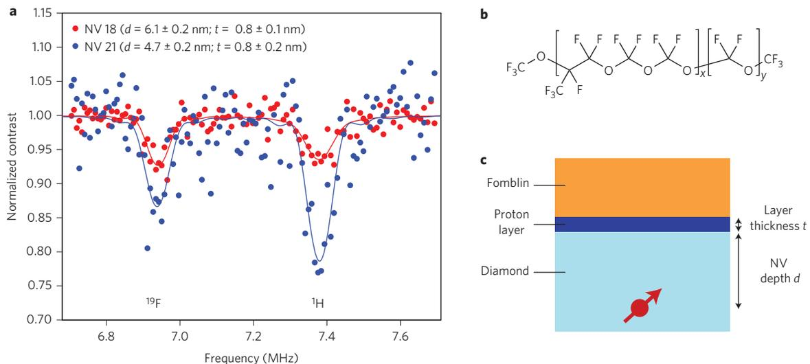
**Figure 5 | Determination of surface proton layer thickness.** **a**, NMR signal from Fomblin Y oil on the diamond surface measured with two NV centres separated by ~5 μm. NV depths are presented, as calculated from the lineshape model (see Supplementary Methods). **b**, Chemical structure of Fomblin Y oil. **c**, Description of the hypothesized sample structure resulting from Fomblin Y oil floating above a thin layer of adsorbed hydrocarbons or water on the diamond surface.
