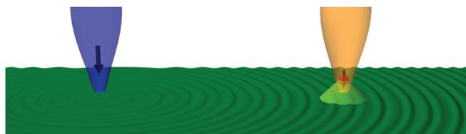
FIG. 1. (Color online) Source-probe measurement setup. The magnetized source (blue cone with an arrow) excites the medium (green). The spin density excitations (pictured as waves) traversing the medium are detected by the probe containing an NV center (red sphere). The probe collects the signal from the magnetization underneath (light green).
